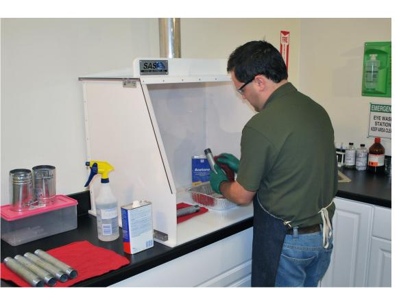
Figure 7. Chemical Fume Hood, a Local Exhaust Ventilation Method used as a control strategy https://www.google.com/url?sa=i&url=https%3A%2F%2Fwww.sentryair.com%2Fblog%2Findustryapplications%2Fchemical-solvents%2Freducing-hazardous-exposure-to-organic solvents%2F&psig=AOvVaw3OPTumUeRIQHvfV9j0htM7&ust=1711901008449000&source=images&cd e&opi=89978449&ved=0CBQQjhxqFwoTCKDmw7GunIUDFQAAAAAdAAAAAA
