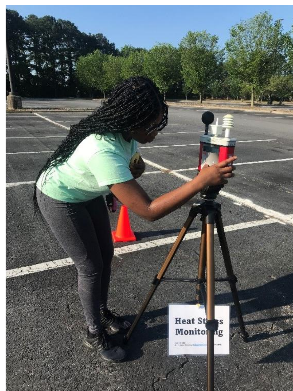
Figure 1: Heat stress monitoring set-up on the parking lot (concrete surface; location 2)
