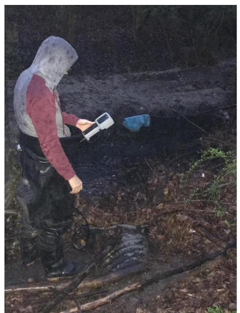
A handheld multi-probe meter was used to measure pH, oxidation reduction potential, temperature, and specific conductance. A flow-probe was used to measure stream velocity and along with the active stream channel dimensions, discharge was calculated. The physicochemical properties of water during stormflow and baseflow were compared. Also compared were the physicochemical properties of water at each location.
