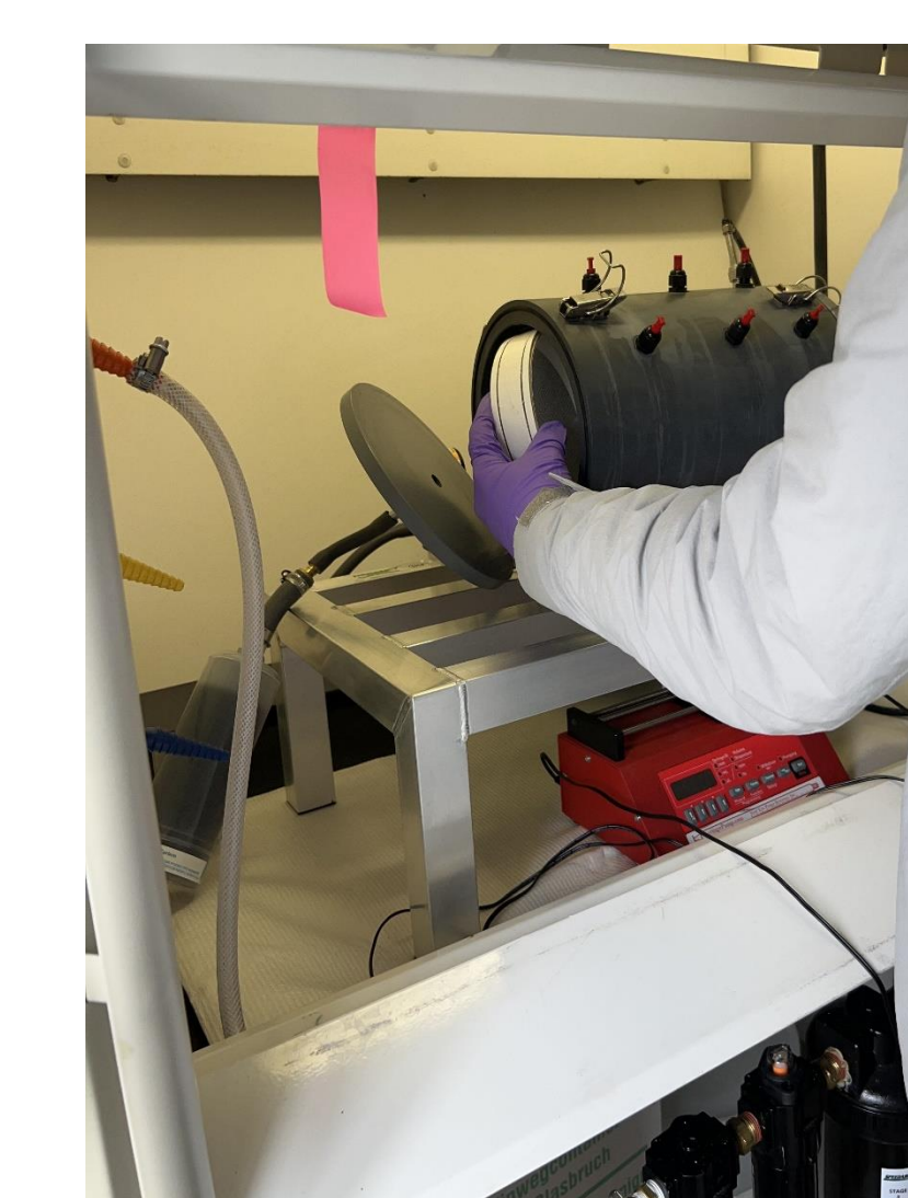
Figure 5. Placing mesh cage into wind tunnel
