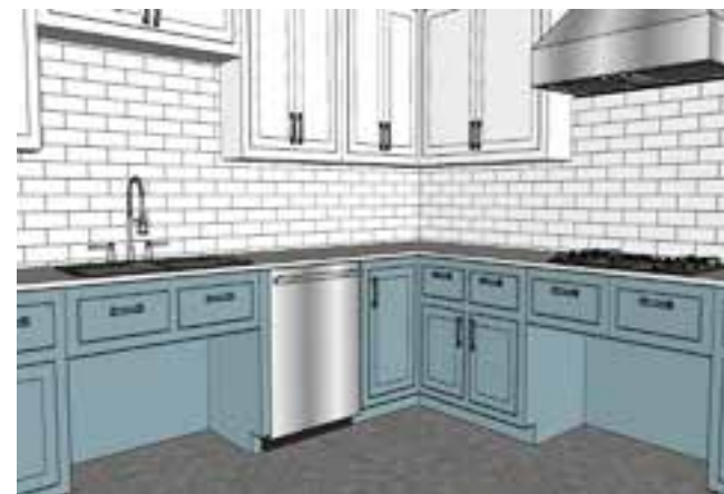
Sink and cook center are open for wheelchair accessibility All counter heights are 34" AFF
