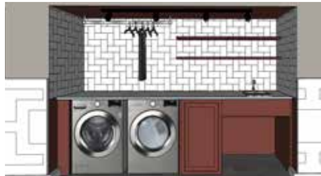
Front load washer and dryer and roll under laundry sink
