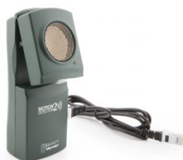
Figure 2.2: (a) Vernier motion sensor and (b) LabQuest2 interface. Images from http://www.vernier.com .
